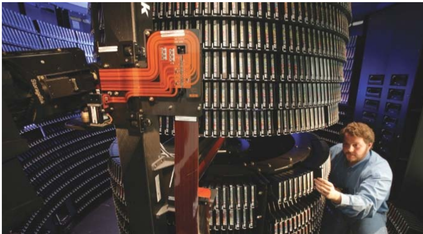
Figure 5. The NCCS massively parallel high-performance storage system (HPSS) data archive allows users to store vast amounts of long-term data.
